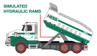
real dump truck, the second piston extends and lifts the truck bed. The 2017 Hess Dump Truck uses a simulated hydraulic mechanism consisting of springs and gears. When the truck bed is horizontal, the springs are compressed. Pushing the appropriate button allows the bed to rise. The gears moderate the lifting force to smooth and slow the movement.
