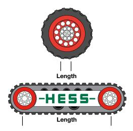
of the two treads and the width of the wheel. Multiplying these numbers will yield the contact area of one wheel.
