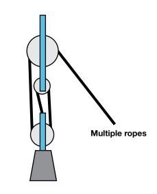
**Pulley MA =** Number of ropes supporting the load
