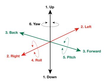
move in more than six different directions: (1) up/down, (2) right/left, (3) forward/back, and the rotating motions of (4) roll, (5) pitch and (6) yaw. Each movement is a degree of freedom. If a joint on a robot arm can move up and down, swing side to side, and rotate, the joint is said to have three degrees of freedom.
