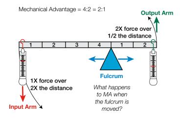
The mechanical advantage of a lever equals the length of the force input arm divided by the length of the output arm. In this example the MA is 2:1 or 2. To measure the forces with the spring scales, one student pulls down on the scale attached to the input arm while another student holds the scale attached to the output arm. Reading the scales reveals the mechanical advantage of the lever.
